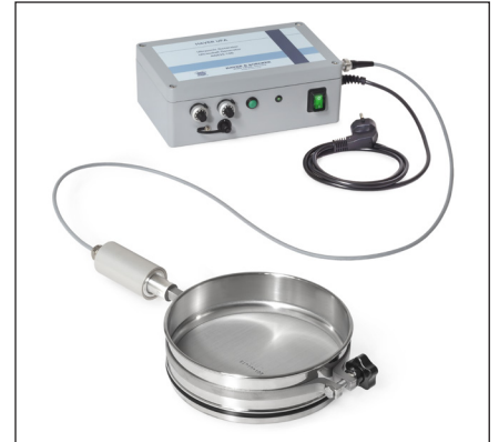
By the use of HAVER UFA the sieving of loose adhesive materials is made possible
