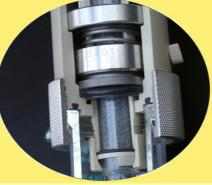
the threepart shaft seal avoids leaks but the stirrer is furthermore height adjustable without any problems
