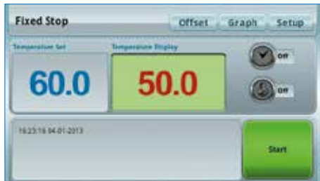
4" Full Touch Screen TFT LCD (Smart-Lab™ Controller)
