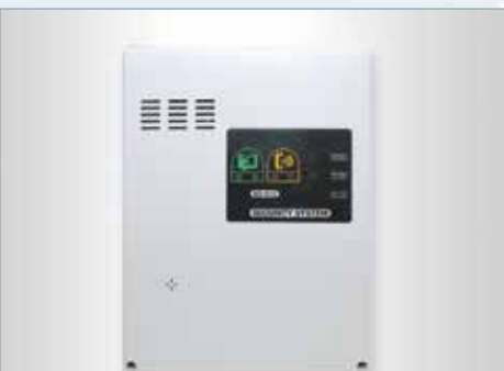
• Remote Wire/Wireless Alarm System (Optional) - Set to be activated when the temperature inside the chamber goes up to -65°C. - Main controller signals to RWAS, if connected, at the alarm status, and then RWAS makes phone calls or send messages. - User could set and store multiple phone numbers and alarm statements.
