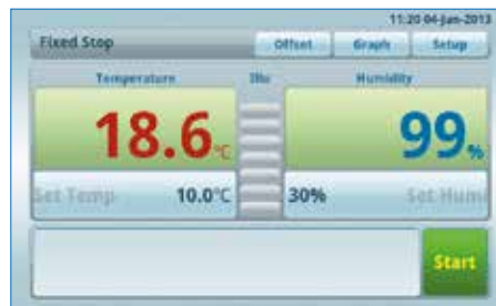
7" Full Touch Screen TFT LCD (Smart-Lab™ Controller)
