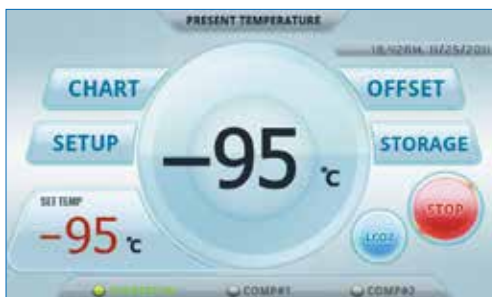
7" Full Touch Screen TFT LCD (Smart-Lab™ Controller)
