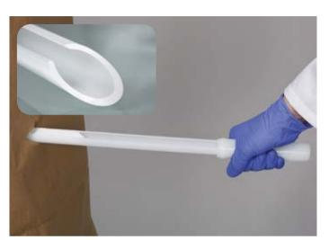
PowderDispo is the ideal disposable sampler for cross-section samples of powdery or slightly cohesive substances. A complete all-layer sample can be taken from bags or smaller containers with the lance.
