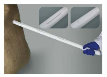
The ZoneDispo disposable all-layer sampler is used in sampling to collect a representative all-layer sample from three different layers. Suitable for free-flowing powders and small-grain granulates. The collected sample can be secured and transported in the closed sampler.
