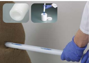
Disposable zone samplers for taking samples from multiple layers of the sample material. Suitable for free-flowing powders and smallgrain granulates. The representative all-layer sample can be emptied directly through the open handle into a sample container.
