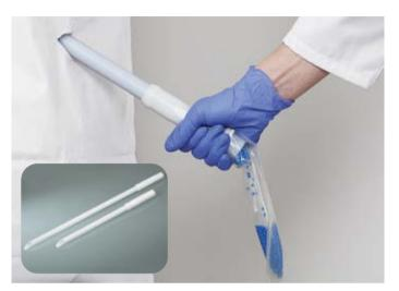
The DispoLance disposable sampler can be used for taking large and small sample quantities quickly and easily, directly from bags. The sampler is suitable for free-flowing powders and small-grain granulates. The DispoLance sampler pierces into the container with the sturdy tip and the sample flows through the open inner tube directly into the container or bag that is held underneath.
